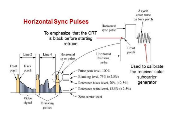
c. <u>Calculate</u> the frequency required for the horizontal and vertical Sync pulses? If 10  $\mu$ s is left for the blanking period, <u>determine</u> the decrease in horizontal resolution of TV transmitter if the video bandwidth frequency is decreased from 4 MHz to 3.5 MHz. (*3 marks*)
