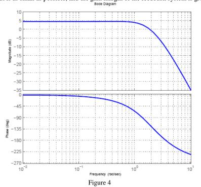
The proportional controller does not change the phase but it does change then gain only We can shift the Bode plot representing the gain 6db and keep a gain margin of at least 5db as shown in figure below
