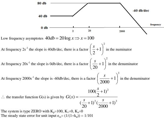
The steady state error for ramp input  $e_{ss} = (1/k_v) = 1/0 = \infty$
