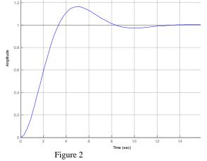
$Mp = \_16\%$ ,  $t_p = \_5$  sec\_,  $t_d = \_1.6$  sec\_,  $t_r = \_3.2$  sec\_, and  $t_s = \_12$  sec\_\_\_\_ for  $\pm 2\%$  tolerance.
