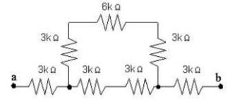
Now the 12  $k\Omega$  in parallel with 6  $k\Omega$  reduces to 4  $k\Omega$ .
