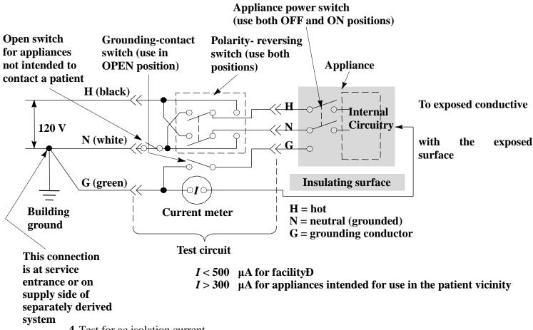
4. Test for ac isolation current
