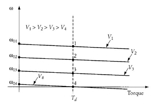
Effect of field voltage on motor speed
