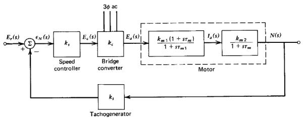
Fig. 6.3 Speed-control loop.
