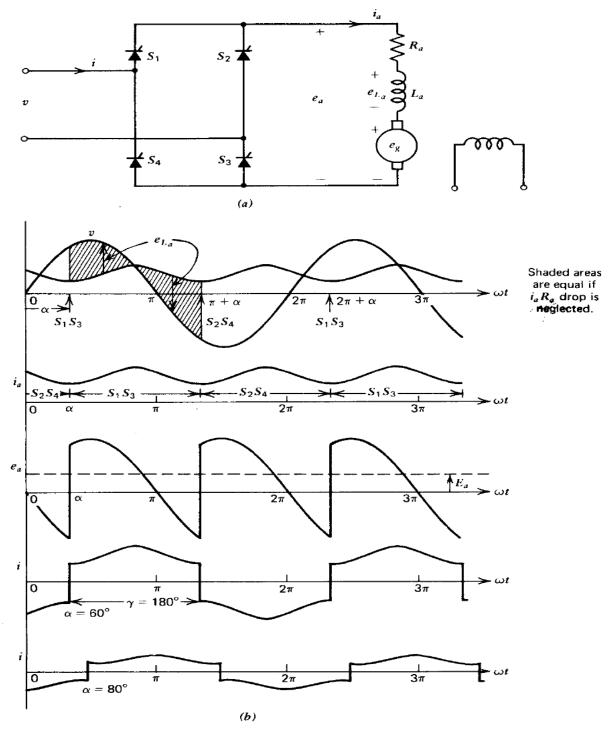
Fig. 2.3 Speed control of a separately excited dc motor by a single-phase full-converter. (a) Power circuit. (b) Voltage and current waveforms for continuous motor current (motor operation). (c) Waveforms for inversion operation.
