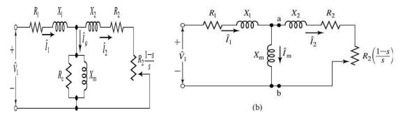
Figure 6.9 Single-phase equivalent circuit for a three-phase induction motor.
