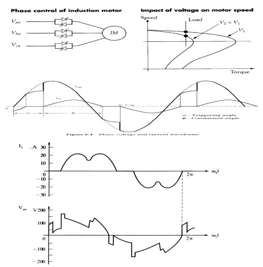
e 6.10 Typical line-current and phase-voltage waveforms of a phase-controlled induction motor drive
