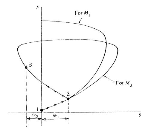
Figure 7 (reflection on pressure deflection diagram) From  $\theta - \beta - M$  curves, for  $M_3 = 1.28$   $\theta_{max} = 6.5$  degrees.
