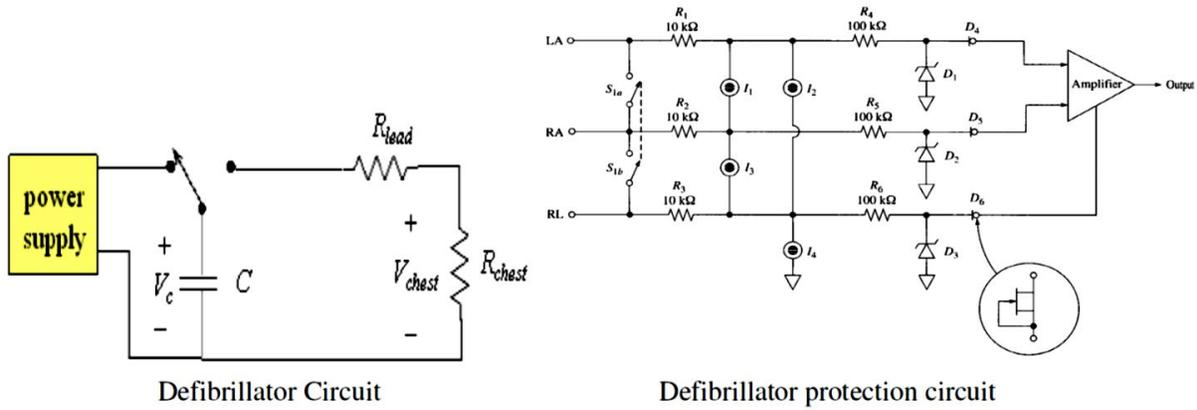
The protection circuit may be only the series resistors or the zener diodes or the neon glow lamps or the FET diodes.
